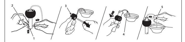
Remove clamp pin (2) and cross pin (1) from downrod. Loosen setscrew in downrod ball (3) until ball moves easily up and down the downrod. Do not remove ground wire (4) from downrod. Slide downrod ball down, exposing cross pin (5). Do not remove ball completely. Remove cross pin and save for later use.
