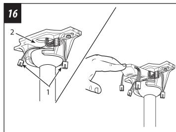
After hanging fan onto the mounting bracket, make sure plug connectors from the ceiling fan and terminal block (1) are moved away from the space located above the downrod ball (2). Slide the remote receiver into the space above the downrod ball as shown.
