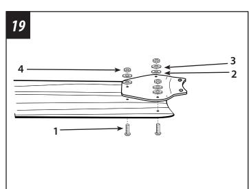
Attach blade brackets to blades using the blade bracket screws (1), rubber washers (2), flat washers (3) and nuts (4). Please screw the screws with a manual scredriver and not with an electric screwdriver!
