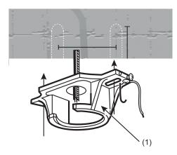
Drill one hole on each side of the supply mains for the expansion anchors. Measure this distance using the oval slots in the mounting bracket (1) as a guide.
