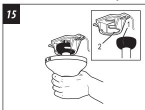
Carefully lift fan assembly onto mounting bracket. Rotate fan until notch on downrod ball (1) engages the ridge (2) on the mounting bracket. This will allow for hands free wiring.
