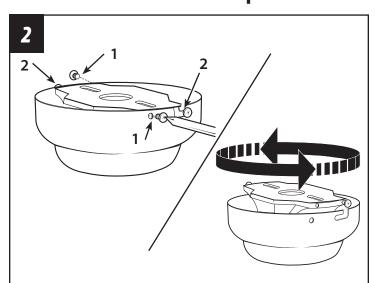
Remove the screws from the two mating holes (1) on the canopy. Loosen (do not remove) the screws in the mating slots (2) on the canopy. Rotate the mounting bracket and remove from the canopy.
