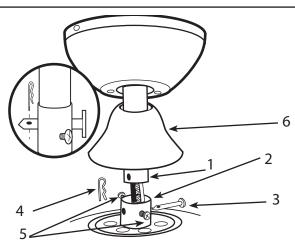
Loose (but do not remove) the set screws from the down rod coupling. Insert downrod (1) into downrod coupling (2). Make sure to align hole in downrod with the hole in downrod coupling. Install cross pin (3) through coupling and downrod. Insert clamp pin (4) into cross pin until it snaps into place. Tighten set screws (5) in coupling. Slide coupling cover (6) over the downrod coupling.
