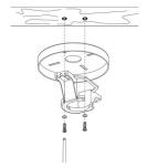
Drill two mounting holes in the ceiling joist and securely screw the mounting bracket to the ceiling using the washers and wood screws provided. The mounting plate should be able to hold a weight of at least 15.9kgs (35 lbs). NOTE - Proper care must be taken when mounting to concrete ceilings. For safe mounting, these ceilings may require stronger screws and plastic plugs or anchors than supplied with the product.
