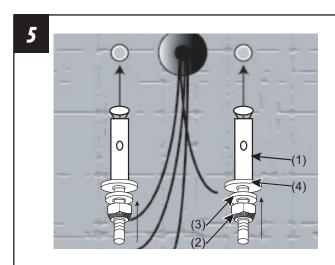
Drive the expansion anchors (1) into the holes. (Note: do not detach hex nut (2), spring washer (3) and metal washer (4) for this step).
