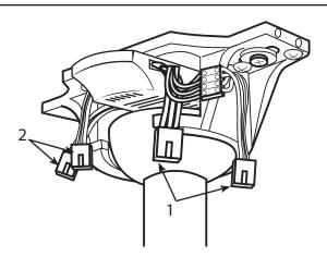
While fan is hanging on bracket, plug 4-pole connector from the mounting bracket into the 4-pole plug connector from the remote receiver (1). Plug the 4-pole plug connector from the fan (2).
