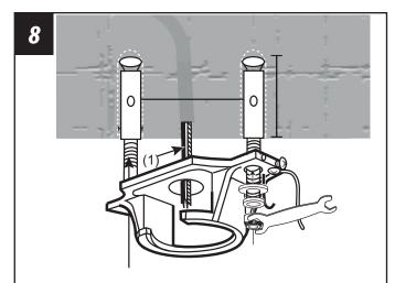
Pull the supply mains (1) through the center of the ceiling, and align the two oval holes in the mounting bracket with the expansion anchors (1), re-install metal washer, spring washer and hex nut, tighten the hex nut until the mounting bracket is fix stably.
